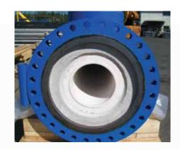
In the cold collector system, the reformed gas is introduced directly from the individual tubes to the transfer line which is located outside the furnace. In this system, special devices are required for connecting the hot parts to the cold collectors. Different versions of this concept are used by Linde Engineering, Haldor Topsoe, Lurgi, Uhde and other engineering companies.
